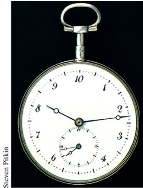
Figure 1.2.1 When the metric system was proposed in 1792, the hour was redefined to provide a 10-hour day. The idea did not catch on. The maker of this 10-hour watch wisely provided a small dial that kept conventional 12-hour time. Do the two dials indicate the same time?
