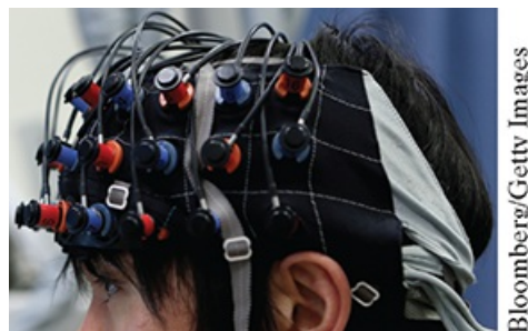
Figure 34.5.4 In functional near infrared spectroscopy (fNIRS), a person wears a close-fitting cap with LEDs emitting in the near infrared range. The light can penetrate into the outer layer of the brain and reveal when that portion is activated by a given activity, from playing baseball to flying an airplane.
