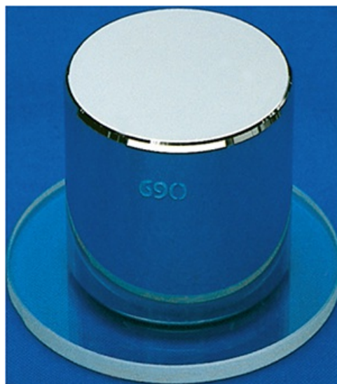
Figure 1.3.1 The international 1 kg standard of mass, a platinum–iridium cylinder 3.9 cm in height and in diameter.
