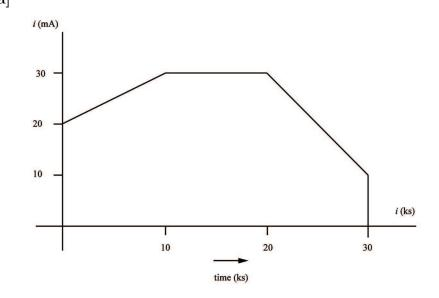
$20 + 1.0 \times 10^{-3} t \text{ mA}, \quad 0 \le t \le 10 \text{ ks};$  $[\mathbf{b}]$  i(t)=10 ks  $\leq t \leq$  20 ks; i(t)30 mA, = $70 - 2.0 \times 10^{-3} t \text{ mA}, \quad 20 \text{ ks} \le t \le 30 \text{ ks};$ i(t)=t > 30 ks. i(t)0, =
