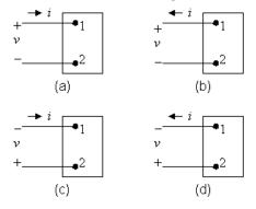
[a] Now we have to match the voltage and current shown in the first figure with the polarities shown in Fig. 1.6. Remember that 4A of current entering Terminal 2 is the same as 4A of current leaving Terminal 1. We get
