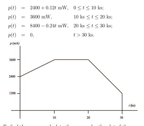
[c] To find the energy, calculate the area under the plot of the power:  $w(10 \text{ ks}) = \frac{1}{2}(10,000)[2.4+3.6] = 25 \text{ kJ};$  w(20 ks) = [10,000][3.6] = 36 kJ; $w(10 \text{ ks}) = \frac{1}{2}(10,000)(3.6+1.2] = 24 \text{ kJ}.$
