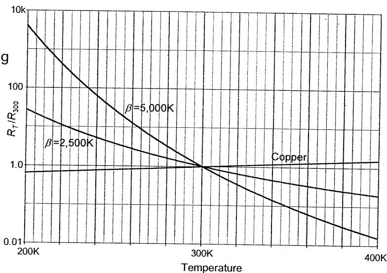
evident from the values of  $R_T/R_{300}$  on a logarithmic scale. The range of values is: 4,160 to 0.0155 ( $\beta = 5,000$ ), 64.5 to 0.125, and 0.61 to 1.39 (copper).
