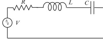
where  $\omega = 2\pi f$ . Calculate  $I$  for the circuit shown if the supply voltage is 80 V,  $f = 50\text{Hz}$ ,  $R = 6\Omega$ ,  $L = 400 \times 10^{-3} \text{ H}$ , and  $C = 40 \times 10^{-6} \text{ F}$ .
