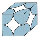
The edge has a length of two times the atom radius, so that the volume of the cube is  $8a^3$ . There is one atom in the structure, which would take a volume of  $\pi a^3$ . Therefore, the atomic packing factor is
