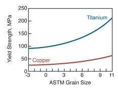
As can be seen, titanium strengthens more with a decrease in grain size (higher ASTM grain size number).
