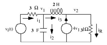
Write the differential equation for each energy storage element.
