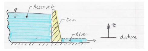
• Engineers select a datum that makes calculations easy. For example, select a datum on the free surface of a river below a dam so that all elevations are positive.
