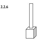
$$W_{total} = (Vol_{container})(\gamma_{water}) + (Vol_{pipe})(\gamma_{water})$$
