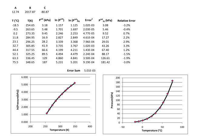
The first and third columns have the data given in the problem statement. The second column has the temperature in K, and the  $4^{th}$  column has the natural logarithm of the vapor pressure data. The fifth column has the result of
